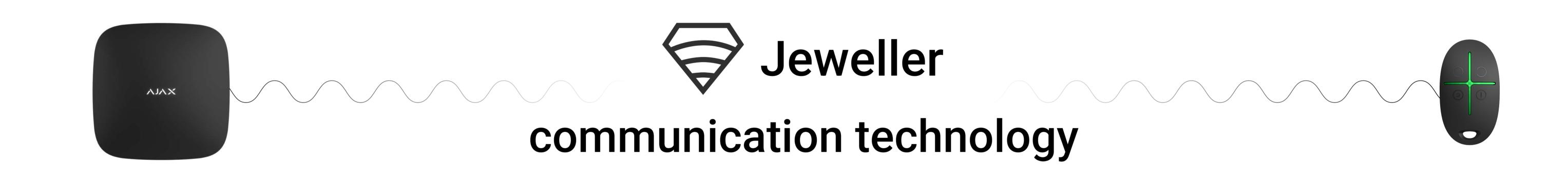
**Jeweller** is a radio protocol for fast and reliable two-way communication between hub (or range extender) and connected devices. The protocol provides a wireless radio communication range with SpaceControl **up to 1300 meters**. This communication range allows using the Ajax security system even on large-scale objects.
